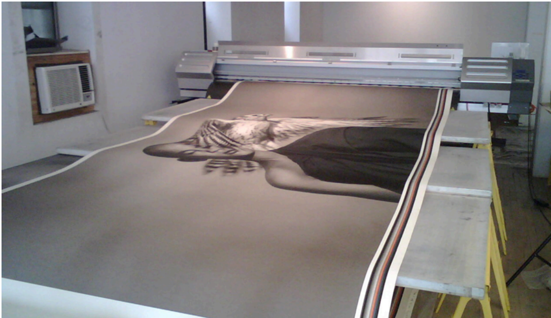
Gregory Colbert prints were produced with Piezography using 110" Roland printer modified to become a 12-ink printer. Credit: Jon Cone
